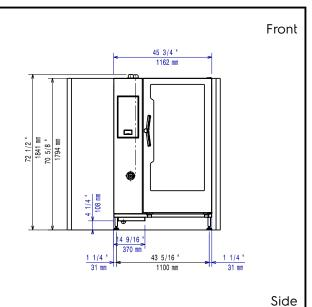
11/16 " 44 mm 44 15/16 " 1141 mm 39 1/2 2 15/16 " 2 11/16 " 1604 mm 63 1/8 3 15/16 " 100 mm 31 5/16 4 13/16 3 1/4 = Electrical inlet (power)
